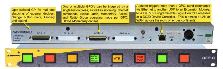
The USP's buttons may be used for control with tally or as a powerful tally display. Define button tally (backlight) colors: Red, Green, or Amber. Set Flashing, Blinking or Solid. Define text legends to be displayed on LCD switch face. Three Font sizes: 1 row of 3 characters, 2 rows of 4 characters, 3 rows of 6 characters!
