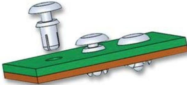
Click-Lock Shank—Place in the hole and press the head. When you hear a snap, the shaft has expanded and the rivet is secured. Pry to remove.
